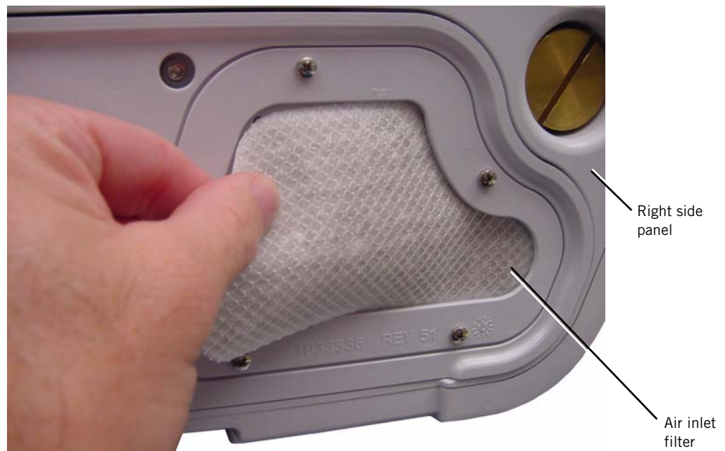
Figure 7-2: Removing the Air Inlet Filter
