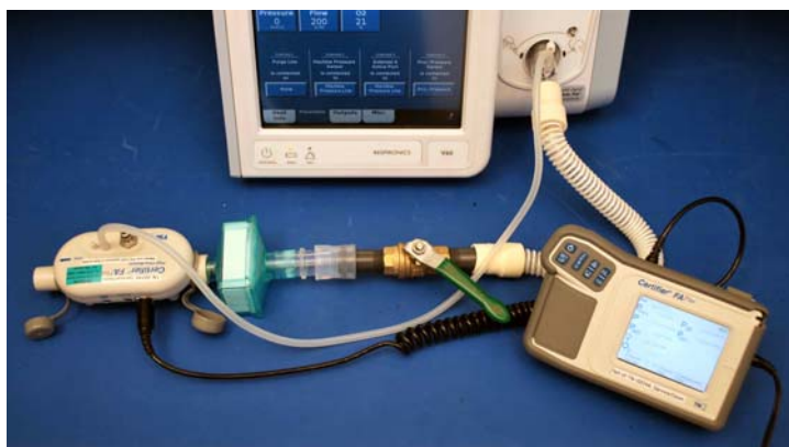
Figure 8-17: Air Delivery Test Configuration
