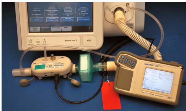
Figure 8-18: Air Flow Accuracy Test Configuration
